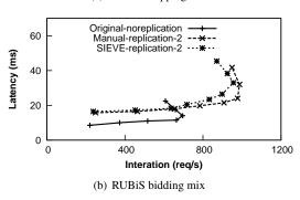
Figure 7: Throughput-latency graph with two replicas.
