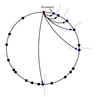
Figure 2.3: Each Chord node divides the address space in exponentially growing areas. The first existing node in each of these areas is called a virtual neighbor and acts as a shortcut to this area.
