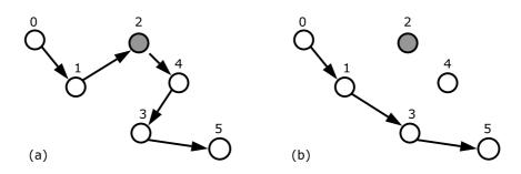
Figure 3.2: Optimization prunes current node from path
