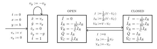
(a) Bouncing ball. (b) RC circuit.
