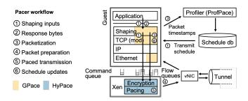
Figure 3: Pacer architecture and workflow.
