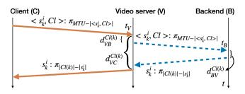
Figure 4: Traffic shaping in video service.  $s_k^i$ :  $k^{th}$  segment of  $i^{th}$  video. Cl: cluster id of the video with segment  $s_k^i$ . |X|: length of payload X.  $\pi_L$ : padding bytes of length L.  $t_V$ ,  $t_B$ : arrival time of incoming request.  $d_{VB}^{Cl(k)}$ ,  $d_{BV}^{Cl(k)}$ ,  $d_{VC}^{Cl(k)}$ : initial delay for  $k^{th}$  segment in cluster Cl. In a **local** setup, shaping is done only on the paths shown by solid arrows.
