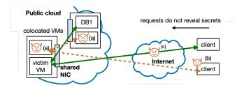
Figure 1: The adversary can (a) colocate with victim's VM or backend services in the Cloud, (b) control clients of its own VMs, and (c) use cross-traffic between any pair of these to infer the shape of the victim's traffic at shared network links.
