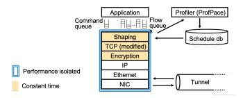
Figure 2: Cloaked tunnel (one endpoint)
