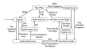
Figure 1: State machine description of an event loop
