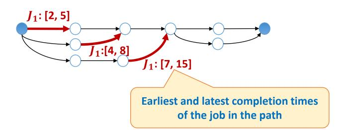
Best-case response time = min {completion times of the job} = 2 Worst-case response time = max {completion times of the job} = 15
