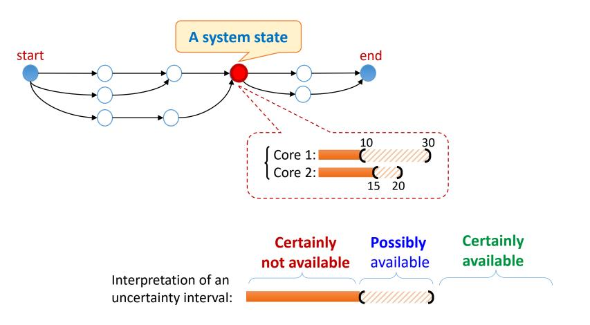
A path aggregates all schedules with the same job ordering A vertex abstracts a system state and an edge represents a dispatched job A state represents the finish-time interval of any path reaching that state
