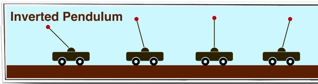
Specification: Mass 0.5 kg, length 0.20 m, period 10 ms **Design:** Current iteration is skipped  $\mapsto$  Use previous iteration parameters Asymptotically stable with at least 76.51% successful iterations\*
