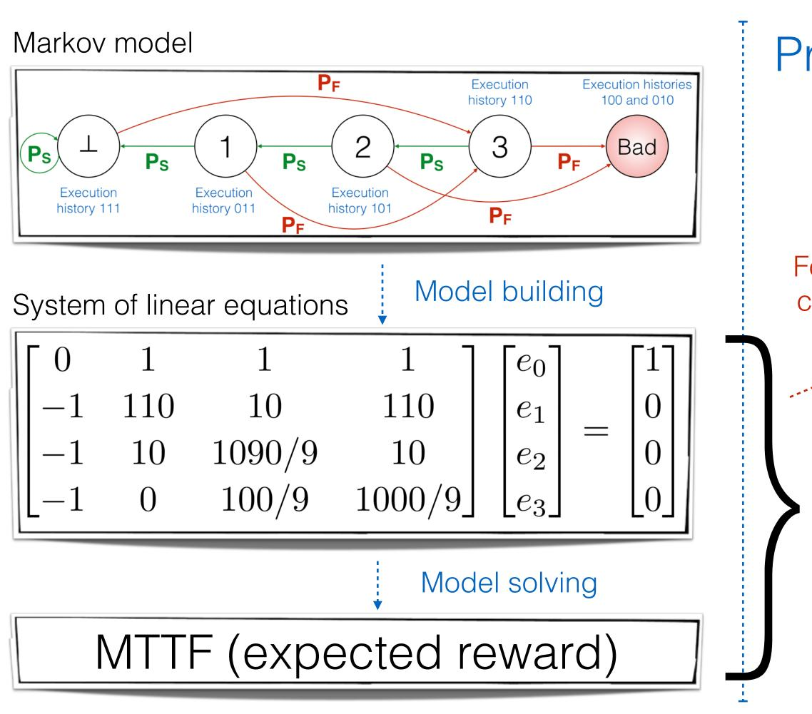
Probabilistic model checking (PRISM under the hood)
