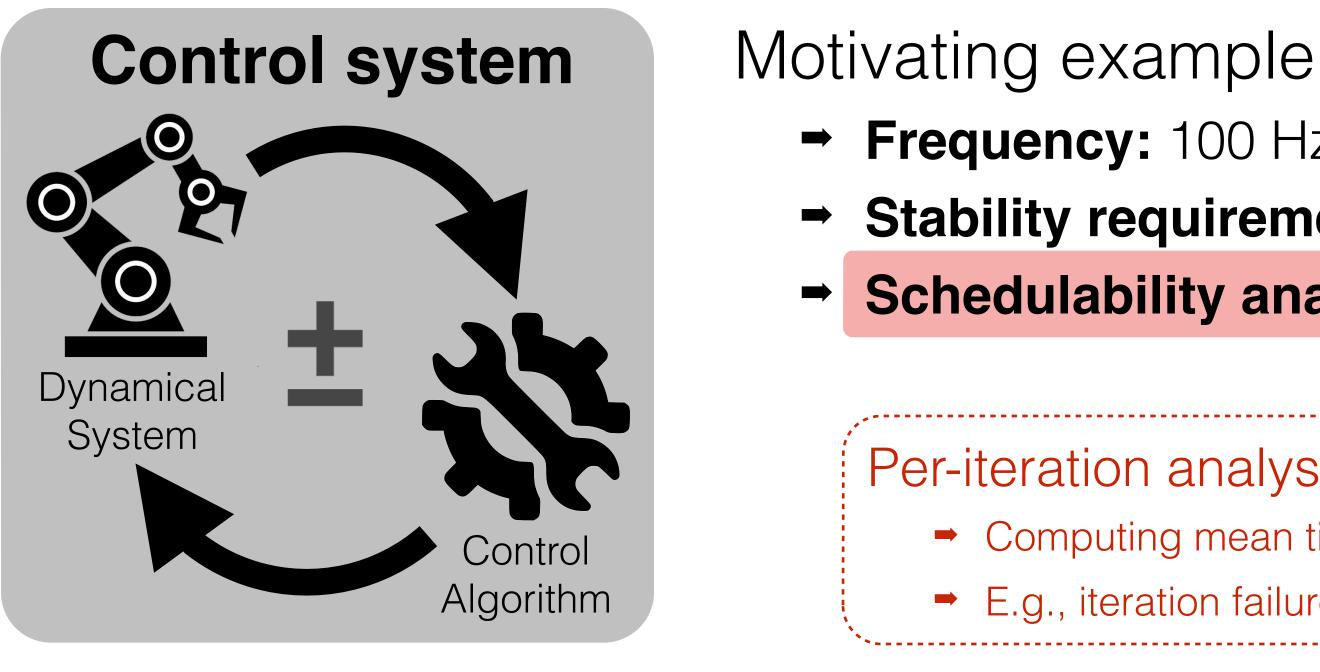
Explicitly accounting for the stability requirements Not trivial anymore! Yields more accurate failure rates E.g., iteration failure probability of  $10^{-10}$  and stability requirement  $\mapsto$  **1.08 x 10<sup>-15</sup> failures / hours**
