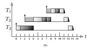
Figure 3: Two example schedules in which three tasks share two local resources (only initial jobs shown, deadlines omitted). The priority ceiling of  $\mathcal{R}_1$  is two, and the priority ceiling of  $\mathcal{R}_2$  is one. (a) PCP schedule. (b) SRP schedule.
