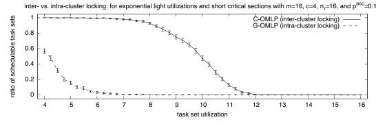
(a) Applying a global locking protocol within each cluster fails if clusters are small
