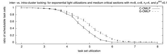
(b) Under global scheduling (m = c), the global mutex protocl is not limited by partitioning constraints
