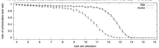
RW vs. mutex: for exponential medium utilizations and short critical sections with m=16, c=1, n<sub>r</sub>=16, p<sup>acc</sup>=0.40, and p<sup>write</sup>=0.2
