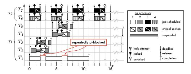
Fig. 3 Seven tasks sharing two resources ( $\ell_1$ ,  $\ell_2$ ) across two two-processor clusters under C-EDF scheduling (the digit within each critical section indicates which resource was requested)
