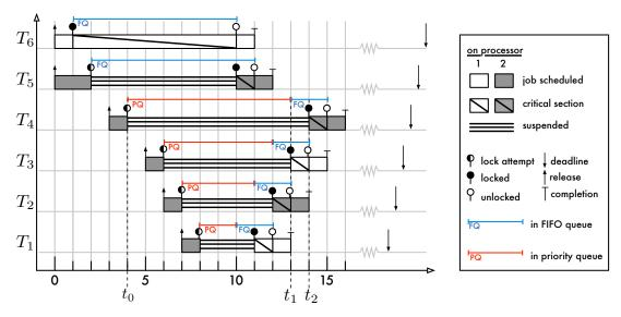
Fig. 10 OMLP mutex protocol for global scheduling under G-EDF for six tasks sharing one resource on m = 2 processors
