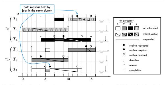
Fig. 7 Six tasks sharing two instances of one resource across two two-processor clusters under C-EDF scheduling (priority donation does not occur in this particular example)
