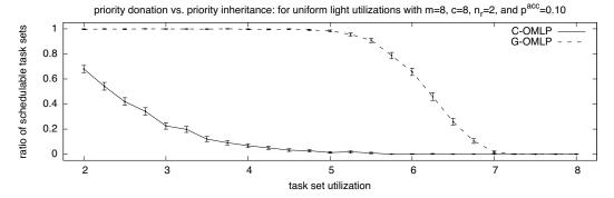
(a) Schedulability is low under the clustered OMLP because urgent tasks are not isolated from long critical sections
