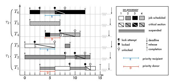
Fig. 5 Six tasks sharing two serially-reusable resources across two two-processor clusters under C-EDF scheduling (the digit within each critical section indicates which resource was requested)
