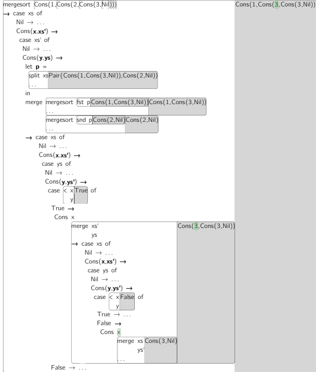
Figure 3. Outermost merge phase of mergesort.
