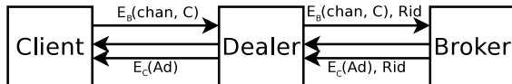
Figure 6: Message exchange for Pub-Sub ad dissemination. E_x(M) represents the encryption of message M under key x . B is the public key of the broker. C is a symmetric key generated by the client for only this subscription.
