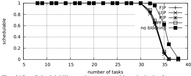
Fig. 815. Schedulability under preemptable spin locks for m = 8 , U = 0.2n , 4 resources, rsf = 0.25 , N^{max} = 1 , and medium critical sections. The schedulability of the considered non-preemptable lock types in this configuration is shown in Fig. 805.
