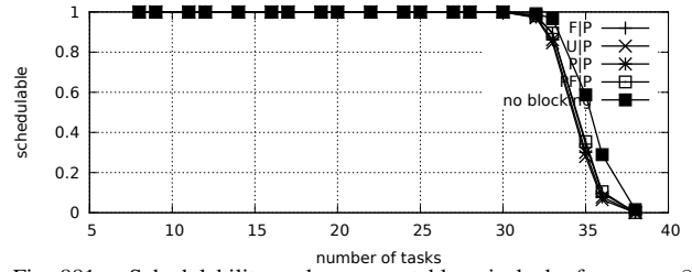
Fig. 881. Schedulability under preemptable spin locks for m = 8 , U = 0.2n , 4 resources, rsf = 0.4 , N^{max} = 2 , and short critical sections. The schedulability of the considered non-preemptable lock types in this configuration is shown in Fig. 871.
