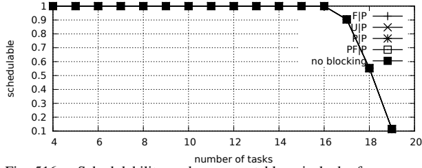
Fig. 516. Schedulability under preemptable spin locks for m = 4 , U = 0.2n , 8 resources, rsf = 0.1 , N^{max} = 2 , and medium critical sections. The schedulability of the considered non-preemptable lock types in this configuration is shown in Fig. 506.
