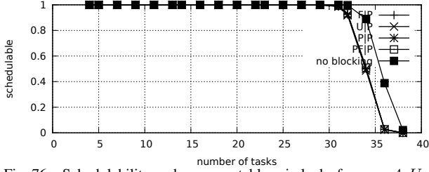
Fig. 76. Schedulability under preemptable spin locks for m = 4, U = 0.1n, 2 resources, rsf = 0.25, N^{max} = 2 , and medium critical sections. The schedulability of the considered non-preemptable lock types in this configuration is shown in Fig. 66.
