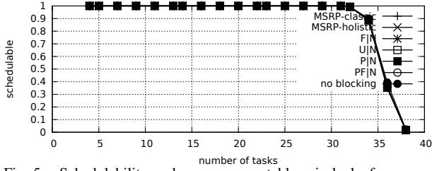
Fig. 5. Schedulability under non-preemptable spin locks for m = 4 , U = 0.1n , 2 resources, rsf = 0.1 , N^{max} = 1 , and medium critical sections. The schedulability of the considered preemptable lock types in this configuration is shown in Fig. 15.
