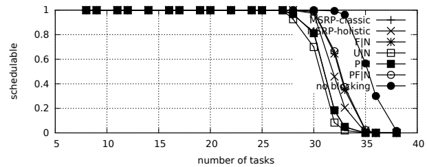
Fig. 1054. Schedulability under non-preemptable spin locks for m = 8 , U = 0.2n , 8 resources, rsf = 0.25 , N^{max} = 15 , and short critical sections. The schedulability of the considered preemptable lock types in this configuration is shown in Fig. 1064.
