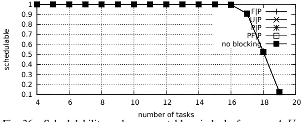
Fig. 36. Schedulability under preemptable spin locks for m = 4, U = 0.2n, 2 resources, rsf = 0.1, N^{max} = 2 , and medium critical sections. The schedulability of the considered non-preemptable lock types in this configuration is shown in Fig. 26.
