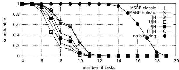
Fig. 688. Schedulability under non-preemptable spin locks for m = 4 , U = 0.2n , 8 resources, rsf = 0.75 , N^{max} = 10 , and medium critical sections. The schedulability of the considered preemptable lock types in this configuration is shown in Fig. 698.
