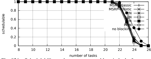
Fig. 826. Schedulability under non-preemptable spin locks for m = 8 , U = 0.3n , 4 resources, rsf = 0.25 , N^{max} = 2 , and medium critical sections. The schedulability of the considered preemptable lock types in this configuration is shown in Fig. 836.
