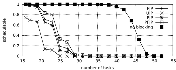
Fig. 1798. Schedulability under preemptable spin locks for m = 16 , U = 0.3n , 16 resources, rsf = 0.25 , N^{max} = 10 , and medium critical sections. The schedulability of the considered non-preemptable lock types in this configuration is shown in Fig. 1788.
