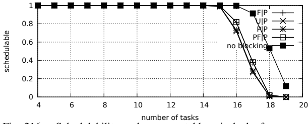
Fig. 216. Schedulability under preemptable spin locks for m = 4 , U = 0.2n , 2 resources, rsf = 0.75 , N^{max} = 2 , and medium critical sections. The schedulability of the considered non-preemptable lock types in this configuration is shown in Fig. 206.
