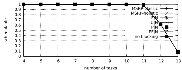
Fig. 534. Schedulability under non-preemptable spin locks for m = 4 , U = 0.3n , 8 resources, rsf = 0.1 , N^{max} = 15 , and short critical sections. The schedulability of the considered preemptable lock types in this configuration is shown in Fig. 544.
