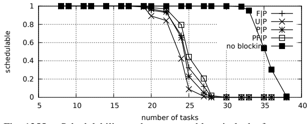
Fig. 1355. Schedulability under preemptible spin locks for m = 8 , U = 0.2n , 16 resources, rsf = 0.4 , N^{max} = 1 , and medium critical sections. The schedulability of the considered non-preemptible lock types in this configuration is shown in Fig. 1345.
