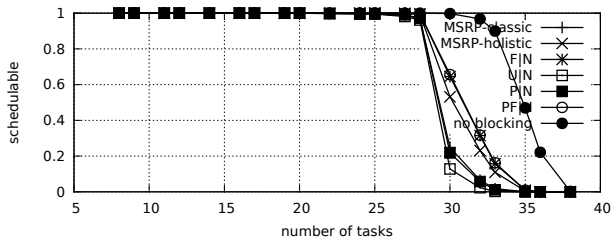
Fig. 1228. Schedulability under non-preemptable spin locks for m = 8 , U = 0.2n , 16 resources, rsf = 0.1 , N^{max} = 10 , and medium critical sections. The schedulability of the considered preemptable lock types in this configuration is shown in Fig. 1238.
