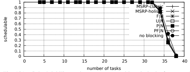
Fig. 131. Schedulability under non-preemptable spin locks for m = 4 , U = 0.1n , 2 resources, rsf = 0.4 , N^{max} = 2 , and short critical sections. The schedulability of the considered preemptable lock types in this configuration is shown in Fig. 141.
