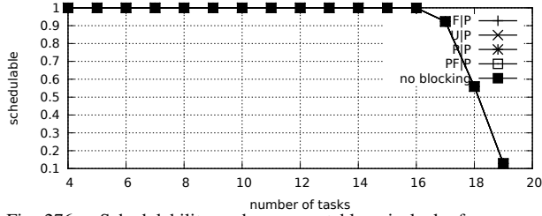
Fig. 276. Schedulability under preemptable spin locks for m = 4 , U = 0.2n , 4 resources, rsf = 0.1 , N^{max} = 2 , and medium critical sections. The schedulability of the considered non-preemptable lock types in this configuration is shown in Fig. 266.
