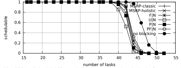
Fig. 2031. Schedulability under non-preemptable spin locks for m = 16 , U = 0.3n , 32 resources, rsf = 0.25 , N^{max} = 2 , and short critical sections. The schedulability of the considered preemptable lock types in this configuration is shown in Fig. 2041.
