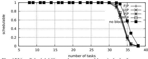
Fig. 1236. Schedulability under preemptable spin locks for m = 8 , U = 0.2n , 16 resources, rsf = 0.1 , N^{max} = 2 , and medium critical sections. The schedulability of the considered non-preemptable lock types in this configuration is shown in Fig. 1226.
