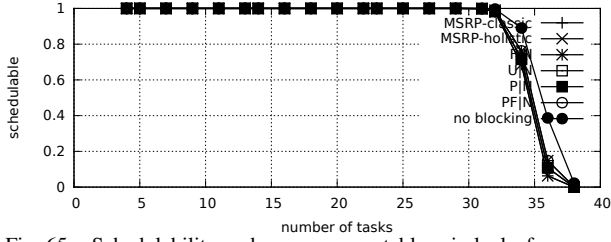
Fig. 65. Schedulability under non-preemptable spin locks for m = 4 , U = 0.1n , 2 resources, rsf = 0.25 , N^{max} = 1 , and medium critical sections. The schedulability of the considered preemptable lock types in this configuration is shown in Fig. 75.
