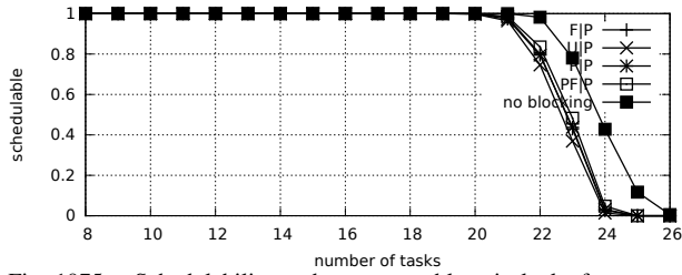
Fig. 1075. Schedulability under preemptable spin locks for m = 8 , U = 0.3n , 8 resources, rsf = 0.25 , N^{max} = 1 , and medium critical sections. The schedulability of the considered non-preemptable lock types in this configuration is shown in Fig. 1065.
